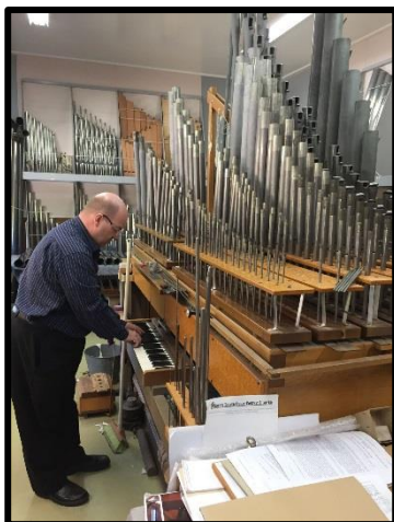
Brett playing some of the new St John's organ Swell pipework on the voicing machine.
