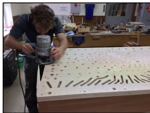
New Great division windchest under construction.
