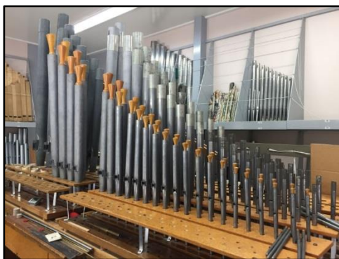
More flute pipes, on the voicing machine.
